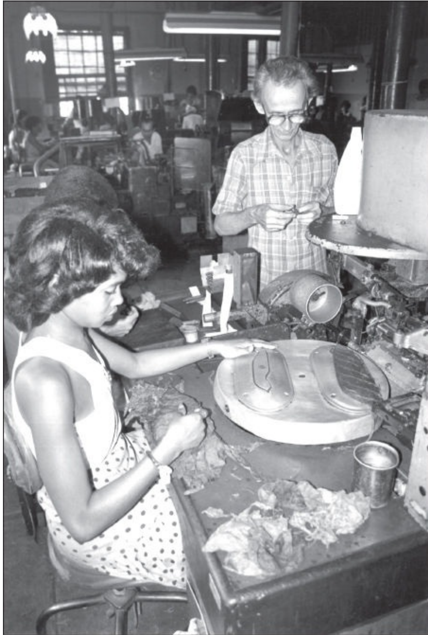
A cigar-making machine at the La Corona factory in Havana. The revolving template is for binder leaf, which will be automatically cut and fed into a bunching machine. In the background, an inspector examines the finished product.
