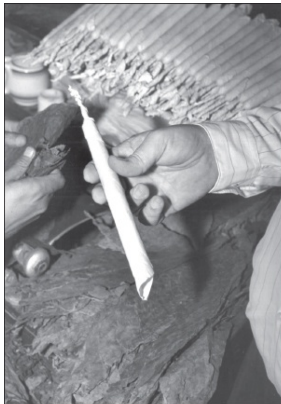
Some wooden molds are not available for special figurado shapes. This Avo (7x36/54) Pyramid, for example, is bunched in a paper mold.
