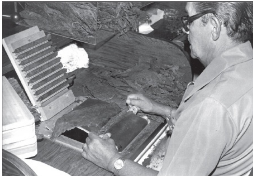
The Lieberman machine, a rubber mat that is rolled by hand, assures overall consistency in bunching. Notice the bunch, near the cigar roller's hands, starting to pick up the binder leaf.
