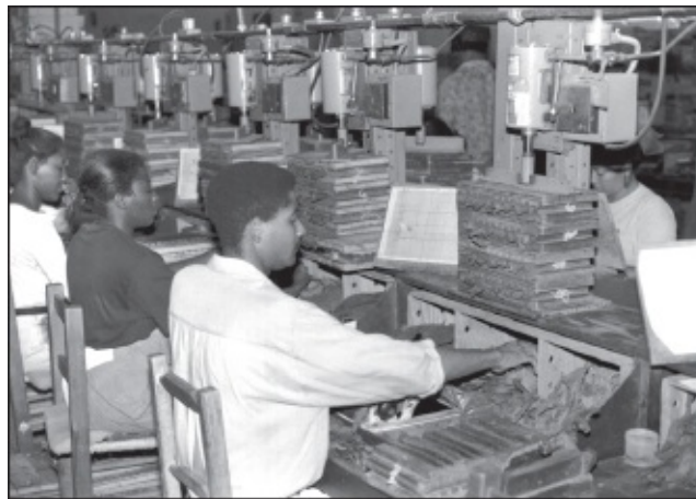
At the Altadis factory, hand rollers work with hydraulic bunching presses located at each station, thus co-mingling updated innovations with traditional cigar rolling methods. In this way, many companies are preserving their handmade craftsmanship while looking ahead to the twenty-first century.
