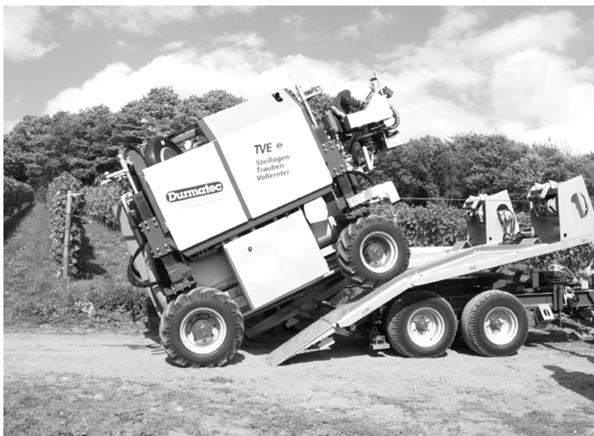
Fig. 15.7 Dumattec cable-drawn steep-slope grape harvester.
