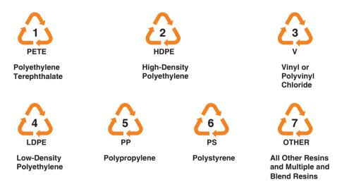
**Figure 8.2** Society of the Plastics Industry (SPI) coding system. (Source: plasticsindustry.org, 2009.)
