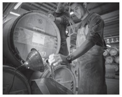
Two cellar workers are shown racking wine through an esquive in the head of a barrel. To facilitate the racking, this esquive has a valve instead of the traditional wooden bung.
