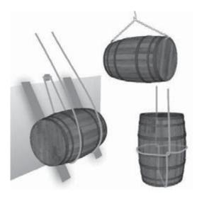
Examples of some of the rigging used to hoist barrels on and off ships and boats.
