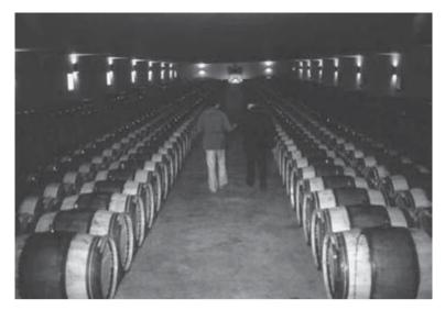
These chateau-style barrels, ageing wine in a wine *chai*, have thinner staves and headboards, requiring the horizon brace on the heads to withstand the pressure. The space between the centre hoops has been stained red to hide any spills.
