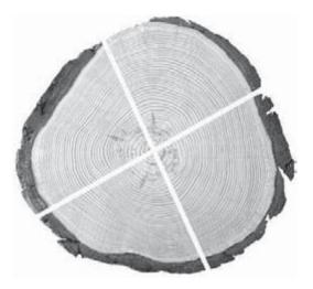
vascular cells, which run up and down a tree. Ideally, the cooper wants the annual rings of the grain visible only at the ends of the staves; otherwise there is the potential for leakage. A winemaker can also check for grain tightness by observing the stave ends.
