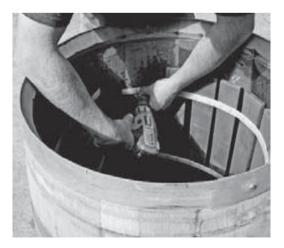
Installing a barrel insert: a set of toasted slats attached to foodgrade plastic rings which hold them in place.
