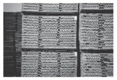
A typical stack of staves drying in a cooperage yard. The staves are angled to allow the rain and snow to drain.
