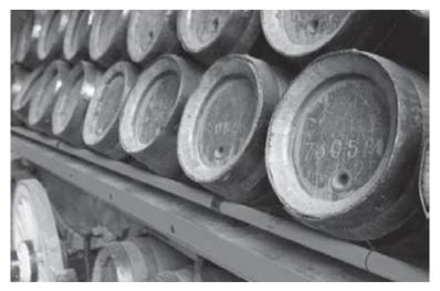
Note the thick staves and wide, strong steel hoops of these beer barrels. The tap would be placed in the small hole in the head of the barrel.
