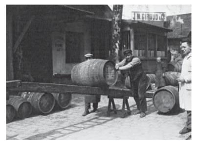
These French workers are loading wine barrels onto a wagon. In the days before forklifts, a ramp was employed to help raise the heavy barrels.
