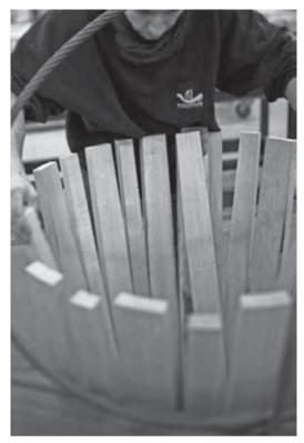
When the staves are assembled, they are splayed outward and resemble a rose. In this photo, the cooper is about to encircle them with the cable, which will be tightened to bring the staves together while they are heated on the bending fire.
