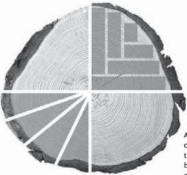
As viewed in this cross-section of a log, the staves are extracted by sawing (upper right) or splitting (lower left).
