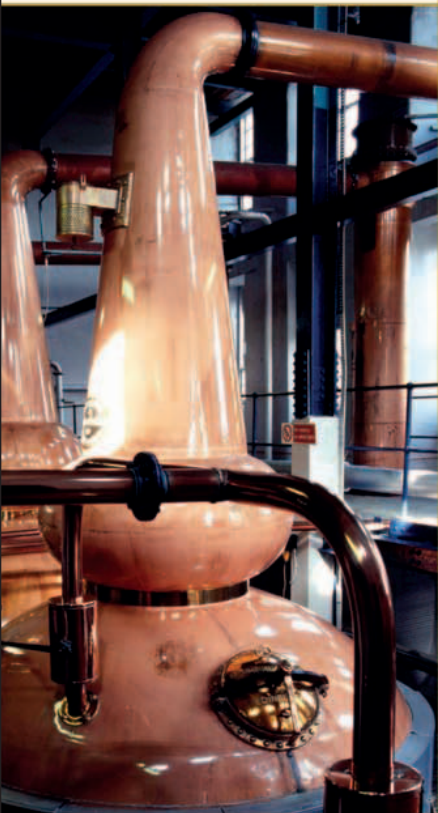
Copper contact The wash produced by fermentation is distilled in either column or pot stills. Stills are made from copper to purify the spirit, with the metal acting as a catalyst to extract sulfur compounds. The size and shape of the still, and how it is operated, will affect the purity and lightness of the spirit.
