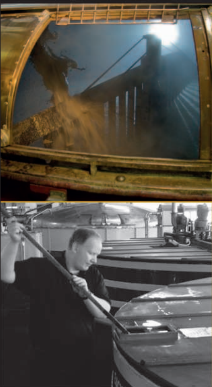
Grist to wash Malt is milled to grist and mixed with hot water in a mash tun to extract the soluble sugars and produce the wort. The wort is then fermented with yeast in brewing vessels called washbacks.
