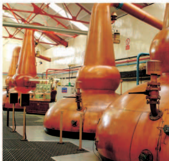
Direct-fired copper pot stills , the largest in Speyside, help to produce a characterful malt.
