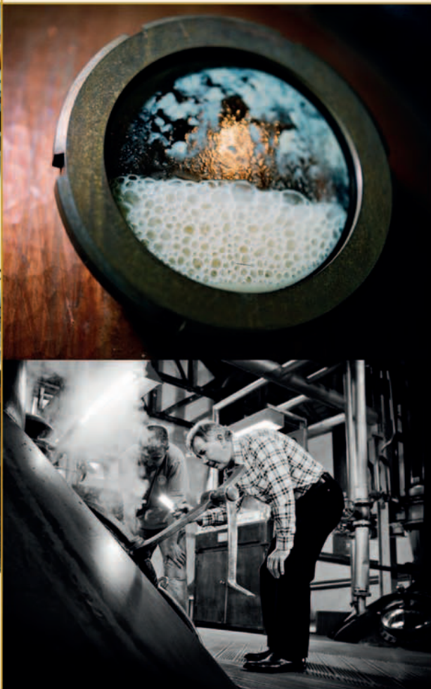
Copper contact The wash produced by fermentation is distilled in either column or pot stills. Stills are made from copper to purify the spirit, with the metal acting as a catalyst to extract sulfur compounds. The size and shape of the still, and how it is operated, will affect the purity and lightness of the spirit.
