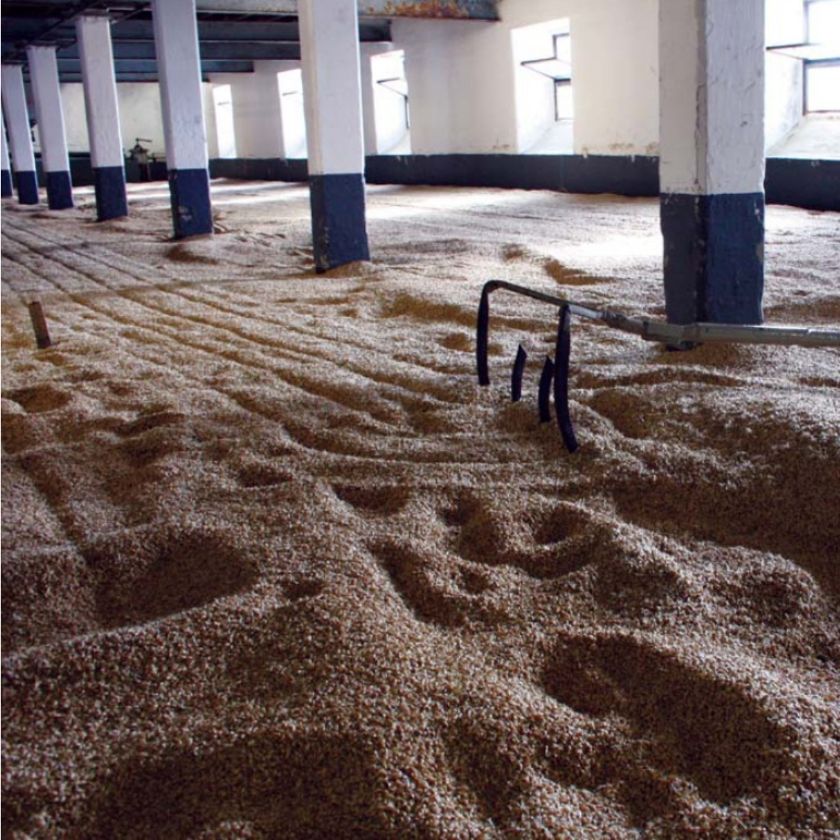
Traditional floor maltings at Laphroaig. Here the moistened barley is heaped up and allowed to start germinating; then gentle fires are lit underneath and it is turned by hand during the drying process.
