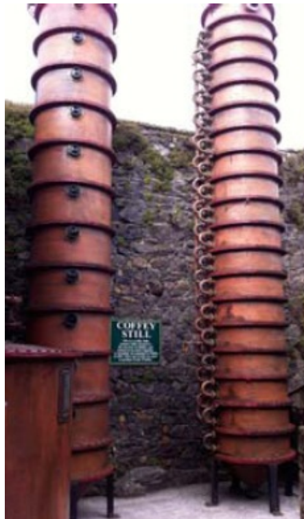
Early Coffey still preserved at Kilbeggan Distillery, West Meath, Ireland. This ingenious heat exchanger, invented two hundred years ago, allows the continuous production of spirit from a mash containing as little as 20 per cent malted barley.
