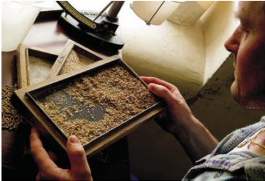
Checking the grist at Glenfarclas. This is malted barley ground into a coarse flour and ready to be turned into 'wash', or unhopped beer.
