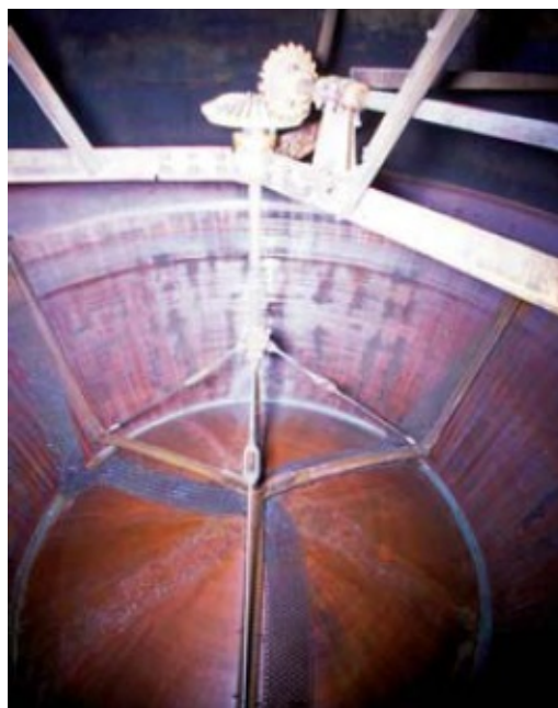
Interior of a still at Glenfarclas. The wash is passed through the still twice. The first pass separates out the worst of the impurities; the second concentrates and refines the spirit to more than 90 per cent ABV.
