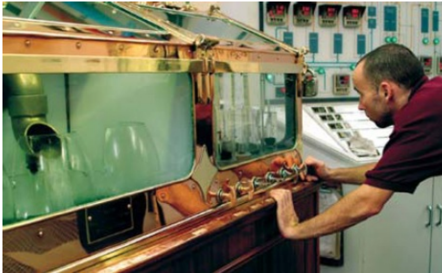
Spirit safe at Glenfarclas. Once the condensed vapour starts running, the stillman has to decide where to start and stop the 'middle cut'. To prevent the removal and sale of spirit before duty is paid, he has to watch the process through a securely locked window.
