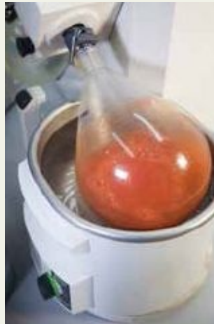
Habanero gin being vacuum distilled at low temperature to produce non-spicy habanero gin.
