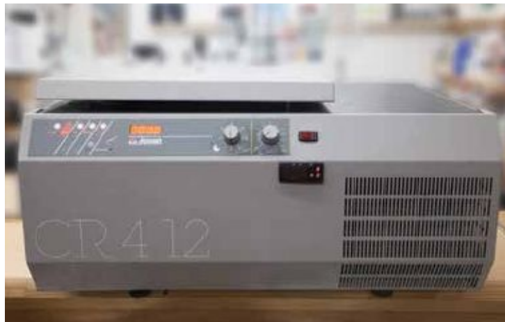
A 3-liter, 4000 g, benchtop, swinging-bucket centrifuge.
