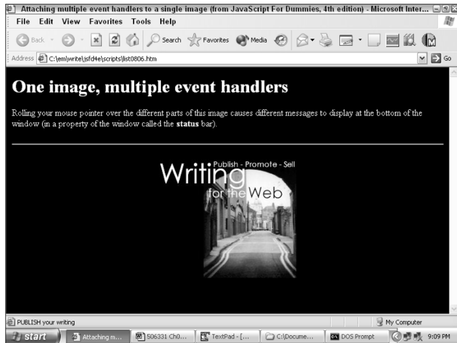
Figure 8-10: The status bar message corresponds to the location of the mouse on a page.
