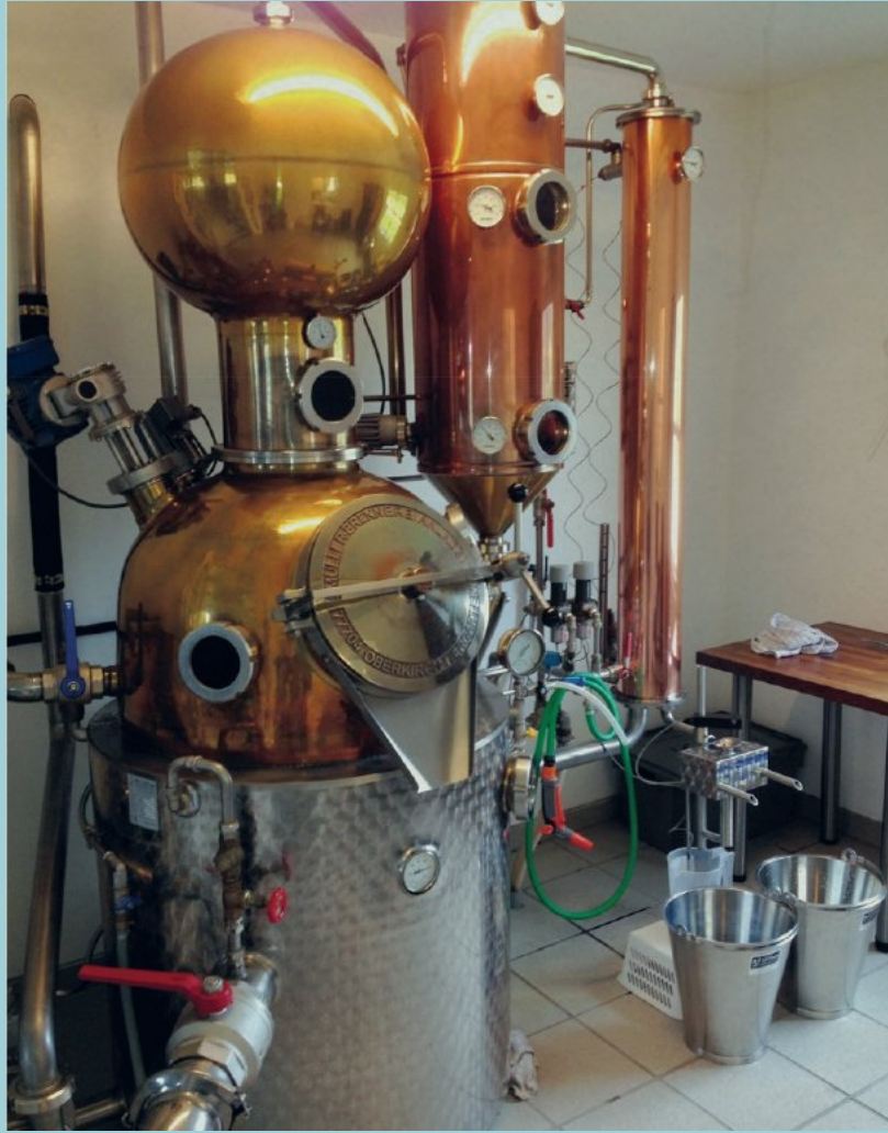
The Mueller pot still at Nordisk is used to triple distil the gin.
