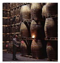
In a palletized warehouse, casks are stored in an upright position, rather than on their sides, so that several at a time can be moved by forklift trucks.
