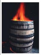
Hakushu Distillery handles the important process of charring its casks at its on-site cooperage.
