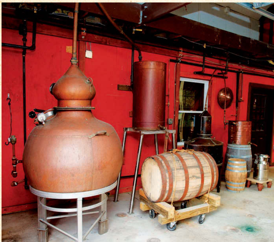
Going into the twentieth century, bourbon distillers mostly used column stills, but many used an easier-to-transport pot still like this one. Today, pot stills are making a slight comeback in bourbon. This one belongs to Tom’s Foolery Distillery in Cleveland, Ohio.
