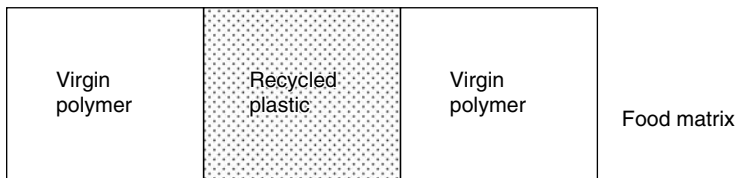
Fig. 17.2 A section through a multilayer package with recycled plastics as a non-food-contact layer (Crockett and Sumar, 1996).
